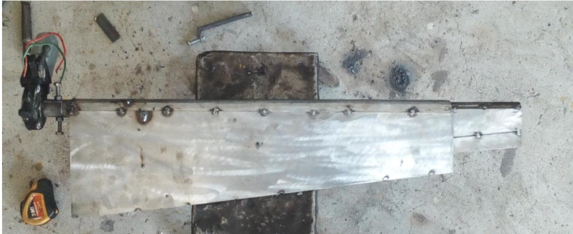
Fig 3. Fabricated model of vari-blade wind turbine blade
